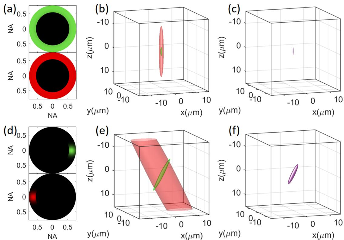
**Figure S1. The numerical simulation of the foci and the chiral SFG point spread function.** First row depicts collinear modality: (a) laser intensity at the objective lens pupil; (b) foci; (c) chiral SFG PSF. Second row depicts noncollinear modality: (d) laser intensity at the objective lens pupil; (e) foci; (f) chiral SFG PSF. The colors green, red, and purple are used to represent wavelengths of 520 nm, 3274 nm, and 448.7 nm, respectively.
