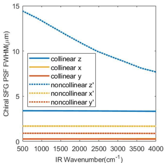
**Figure S2. The dependence of the chiral SFG PSF FWHM on wavelength.** The wavelength of mid-IR beam is tuned to scan across typical vibrational resonance range.
